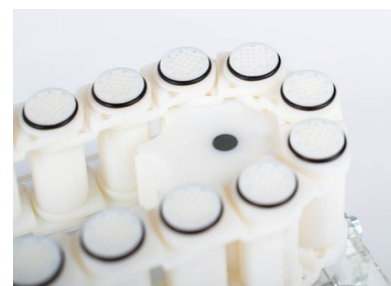
Sterile insect release mechanism that is compatible with UAVs
