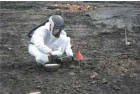
Collecting confirmation samples from the bottom of Sen Lake after excavation (Photo: CDM Smith)
