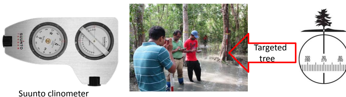
Figure 23: Bearing measurement using Suunto clinometer
