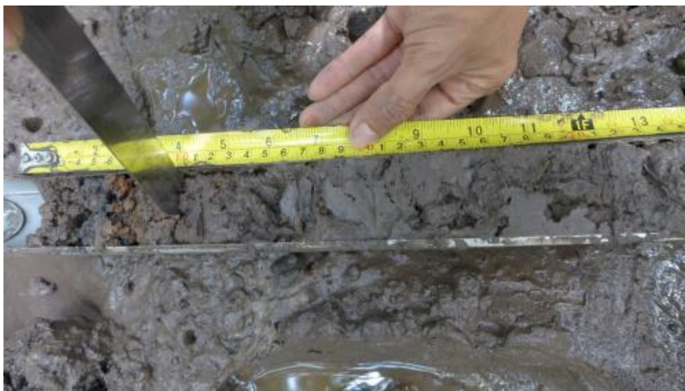
Figure 32: Include the measuring tape when taking photos of soil samples (© Frida Sidik, FAO)
