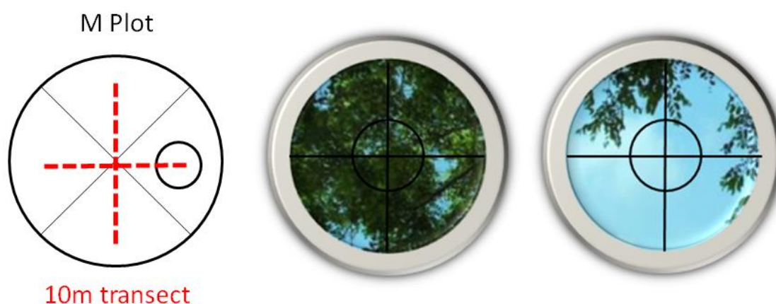
Figure 27: Using the GRS Densitometer to measure the leaf cover on two 10m transects in each subplot
